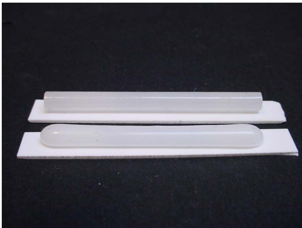
Fig 4: samples of glass before and after the measurement with MISURA LT optical dilatometer.
