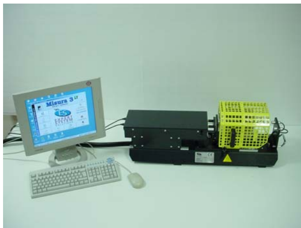
The new MISURA LT horizontal optical dilatometer
