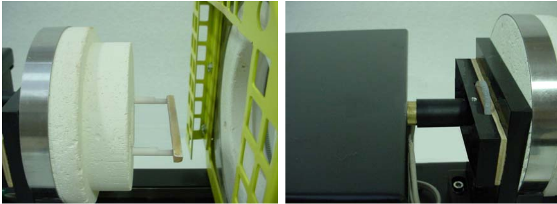
Detail of the no-contact measuring system of the optical flexion meter MISURA FLEX, with sample suspended between two supports 70mm apart.
