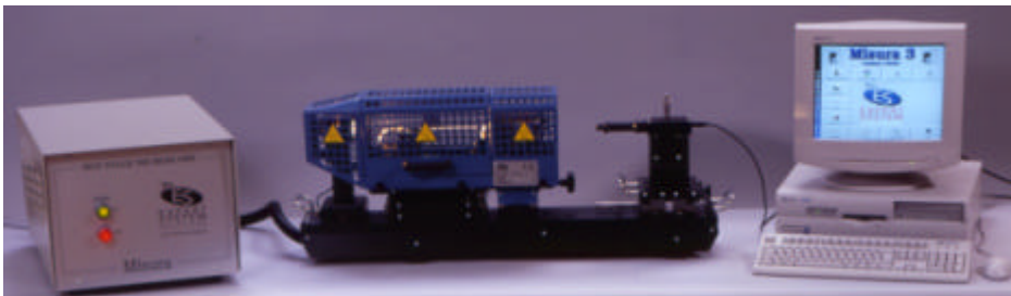
fig. 1: Heating microscope MISURA HSM of Expert System Solutions
