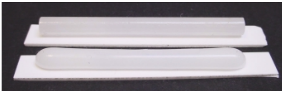
Figure 7. Glass rod specimens before and after the thermal expansion test. After the test, the edges of the specimen are completely rounded.
